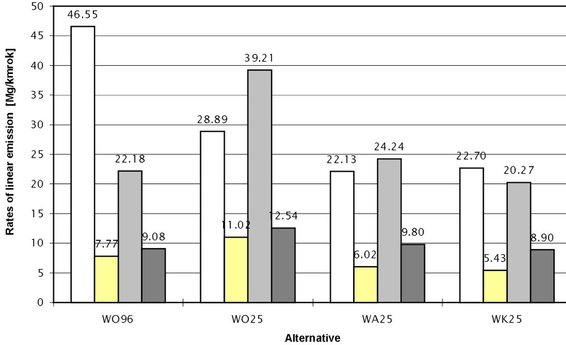
Fig. 4. Rates of linear emissions of CO [Mg/km/year] for three groups of road categories (First column,– roads A, S and GP, second column – other roads G, Z, L and D, third column – urban roads, fourth column – average values) and evaluated alternatives of networks
