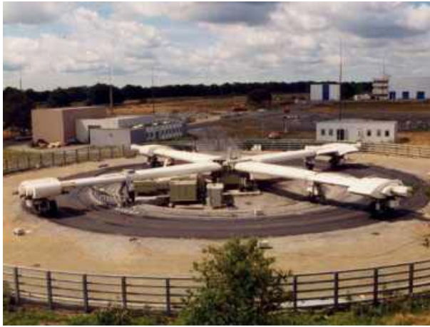
Circular fatigue carousel (diameter 20 m)
