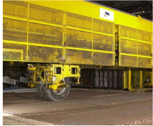
Linear fatigue machine (length 2 m)
